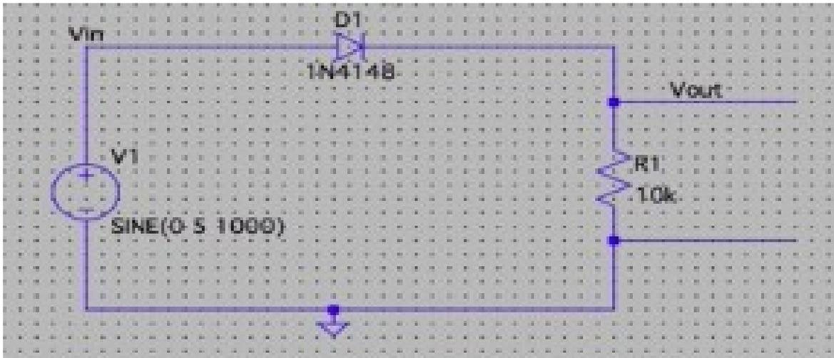
**Step 8.** Simulate Vout when  $V_{in} = 5 \times \sin(2\pi \times 1000 t)$ , or sine wave with amplitude of 5V and frequency of 1 kHz. Copy the simulated graph in your electronic lab notebook. Save the circuit file to submit.
